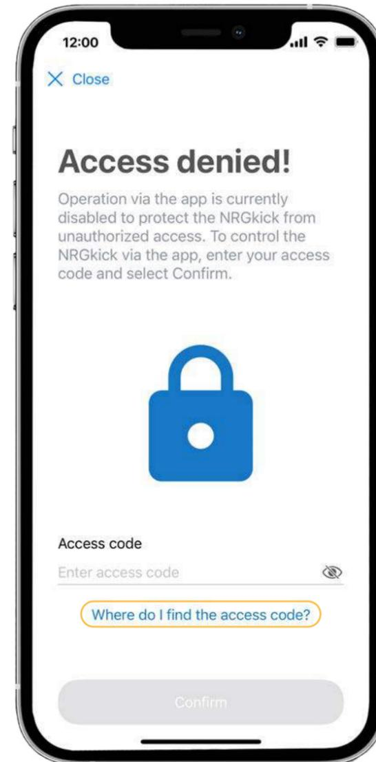
2.2. Enter the access code: The access code consists of the 7 digits before the letter „S“ in the serial number. You will find the serial number on the back of the NRGkick. You can later change the access code [see step 5].
