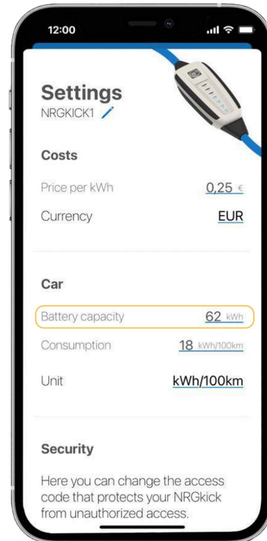
**6.2.** Under „Battery capacity“ you can define the battery size. Slide the setting area down to save the change.
