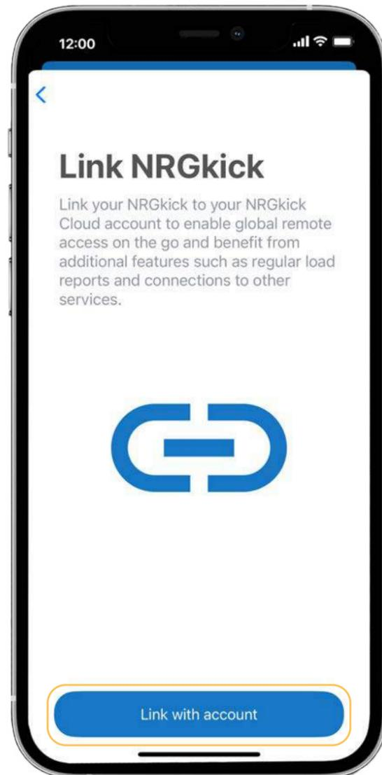
**4.5.** If no cloud account is set up during the initial setup, you can do this at any time. To do this, open the app and get close to the NRGkick (< 10m), as the connection is initially established via Bluetooth.
