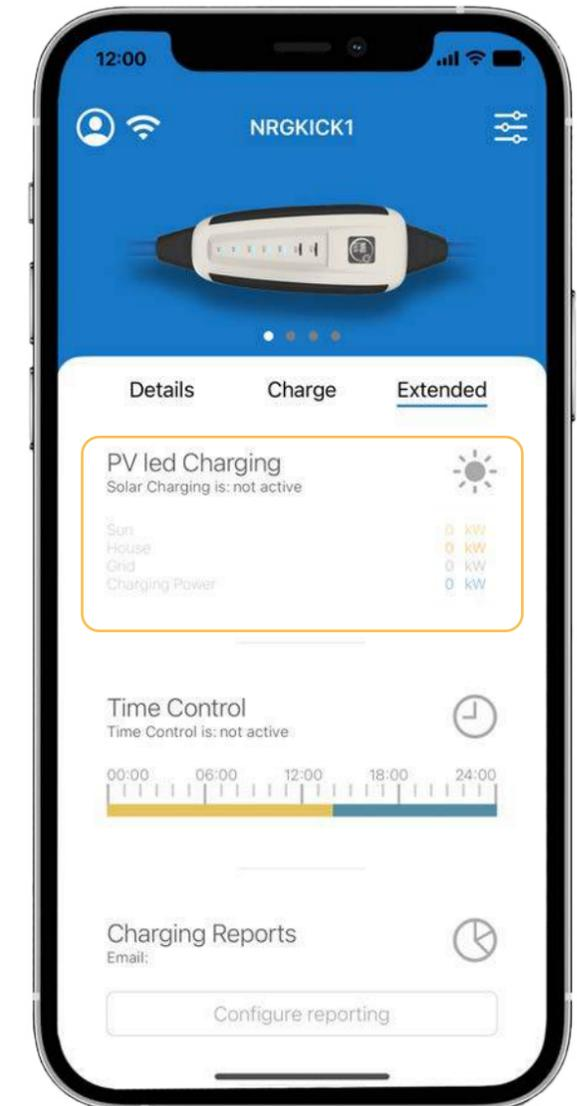
**10.4.** Now you will see the newly enabled „PV-led Charging“ function in the app. By tapping on „PV-led Charging“, you can start the setup.
