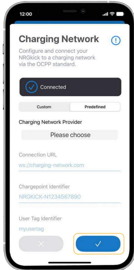
Fill in user ID: Depending on the provider, the user ID is either filled in automatically (as part of the NRGkick serial number) or must be entered manually.
