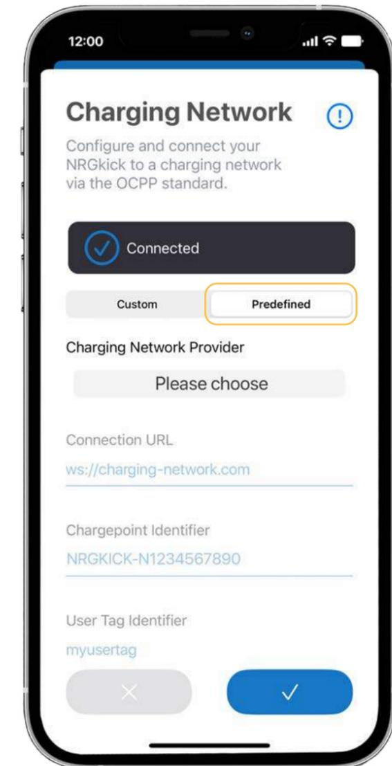
**9.2.** If the charging network partner is permanently integrated, select „Predefined“. Connection URL and charger ID are pre-filled in this case (from components of the NRGkick serial number).
