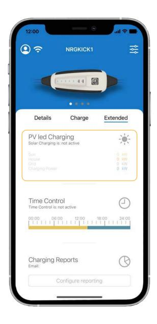
**1.4.** Now you will see the newly enabled "PV-led Charging" function in the app. By tapping on "PV-led Charging", you can start the setup.
